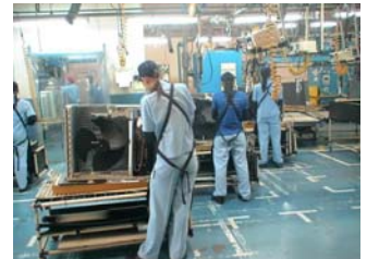
Outdoor unit assembly Yatai (Single cubicle production)
