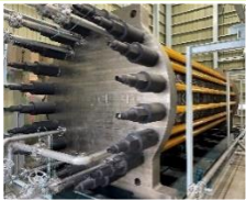
Alkaline water electrolyzer (in operation)
