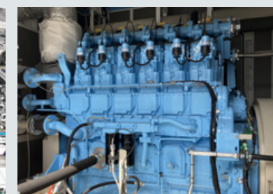
500 kW-class 6-cylinder hydrogen engine (prototype)
