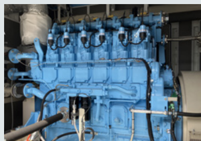
500 kW-class 6-cylinder hydrogen engine (prototype)
