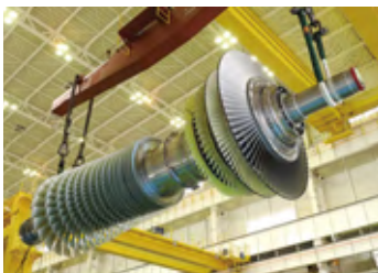
A "J-Series" gas turbine achieved the world's highest turbine inlet temperature 1,600°C, during verification testing. (2011)
