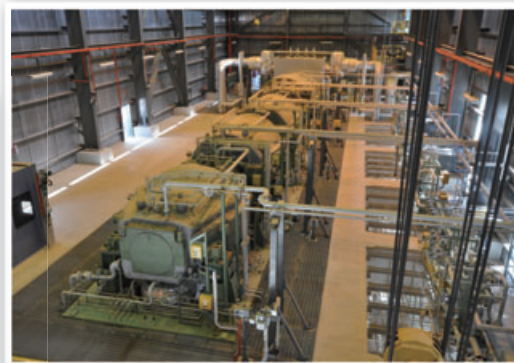
▲ Compressor and mechanical drive steam turbine for world's largest ethylene plant in the UAE
