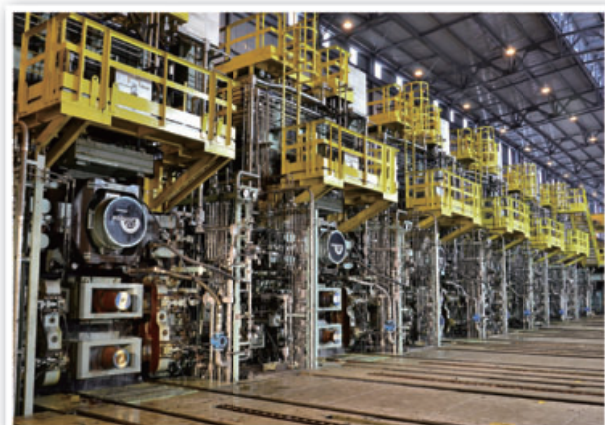
▲ Hot Rolling Mill
