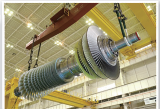
▲ M501J gas turbine
