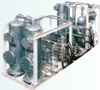
Mobile Unit of Solvent Extraction System for Oil & PCBs* Contaminated-Soil Remediation (*Polychlorinated Biphenyls)
