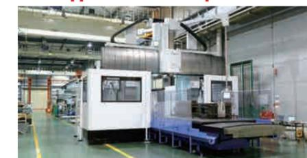
In May 2014, MHI unveiled a new model in its MVR Series of double-column 5-face milling machines, the MVR-Ex. By incorporating an internally cooled main spindle and thermostabilized columns, MHI overcame heat problems and succeeded in enhancing heavy-duty machining and high-precision finishing. MHI is confident this latest model will attract new users and prove popular among existing users.
