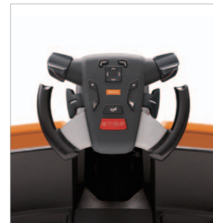
Rapid low level order picker (PS20), one of the red dot winners, is equipped with an ergonomically designed steering wheel that resembles a game controller, making it easier to operate
