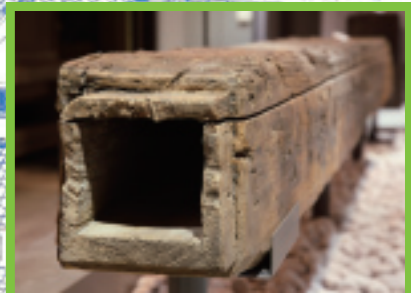
Mokuhi (wooden conduit) This is a wooden square conduit that served as a water pipe. The size and shape varied depending on the place it was used. Some also had round or triangular shapes.
