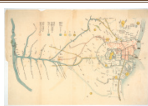
The waterworks of Edo This is a map showing the distribution of the waterworks in Edo around the end of Shoutoku (1711-1715). Water taken from the Tama River was diverted to supply water for farming in its midstream. On entering the Edo of the time, a great network of water pipes would have spread out before one's eyes, as can be seen in this map.
