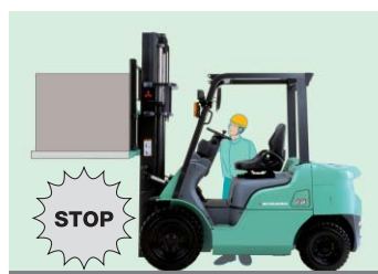
Lift, tilt and travel levers (torque converter vehicle) will not function when the operator is not seated.
