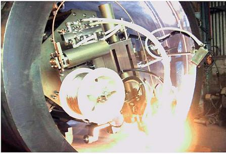
Fig. 6 Remote automatic TIG weld testing performed on inner surface of outlet nozzle mock-up
