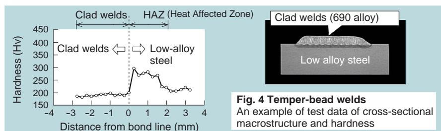
Fig. 4 Temper-bead welds
