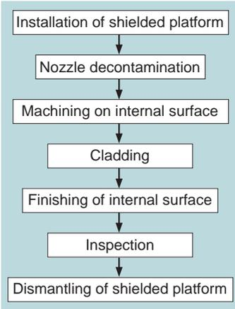
Fig. 5 Work procedure
