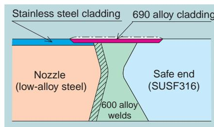
Fig. 2 Profile of clad welds
