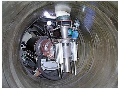
Fig. 7 Decontamination device testing performed on inner surface of outlet nozzle mock-up
