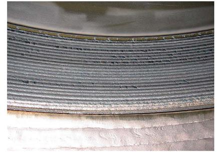
Fig. 9 Actual welding surface (before finishing)
