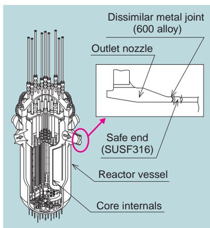
Fig. 1 Reactor vessel outlet nozzle
