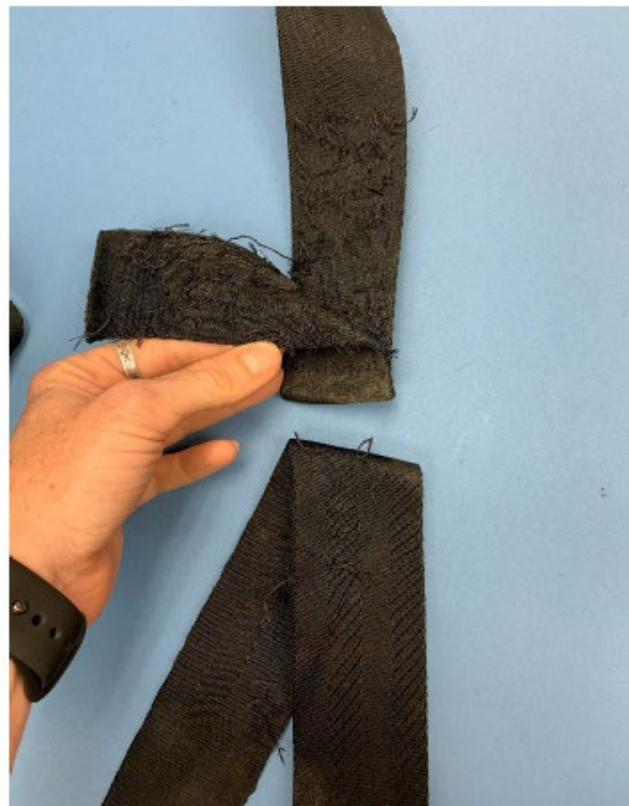
Figure 2 Four-point restraint assembly with separation at shoulder harness Y-junction threading
