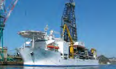
2005 Constructed the deep-sea drilling vessel, CHIKYU, capable of drilling up to 7,000 m below the seabed
