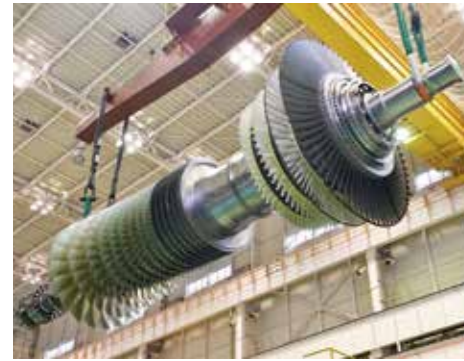
M501 JAC Gas Turbine Rotor
