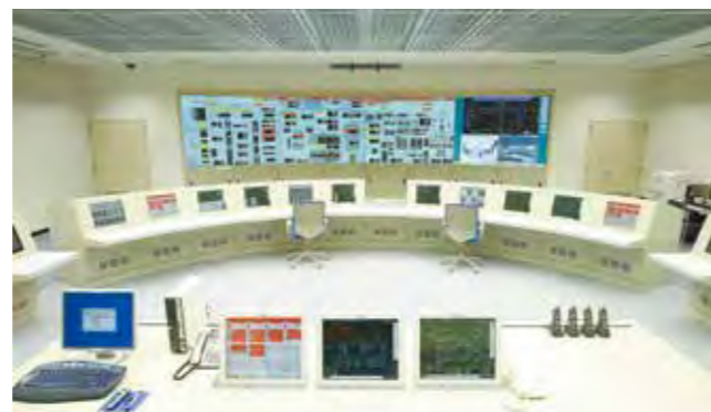
Full-scale Simulator for Operator Training
