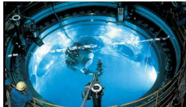
Ultrasonic Testing Equipment for Reactor Vessel (A-UT machine)
