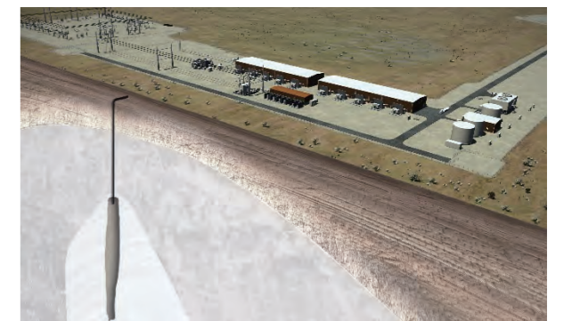
Figure 41 Illustration of hydrogen production and storage plant
