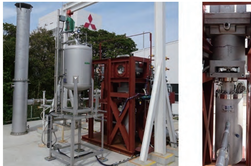
Figure 49 Liquid hydrogen pressure booster pump for hydrogen fueling stations
