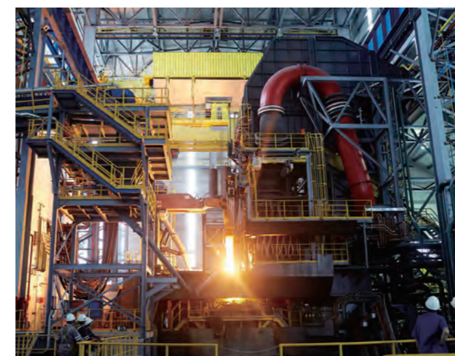
Figure 33 New electric furnace (Quantum EAF)
