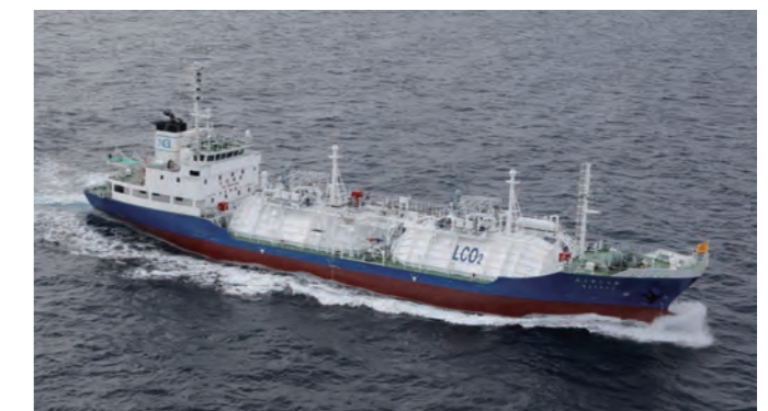
Figure 56 "EXCOOL", a demonstration test ship for LCO 2 transport
