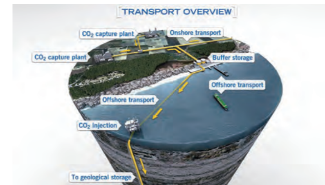
Figure 55 Over view of CO 2 transportation Source: "Fact Sheet: Transporting CO 2 " Global CCS Institute
