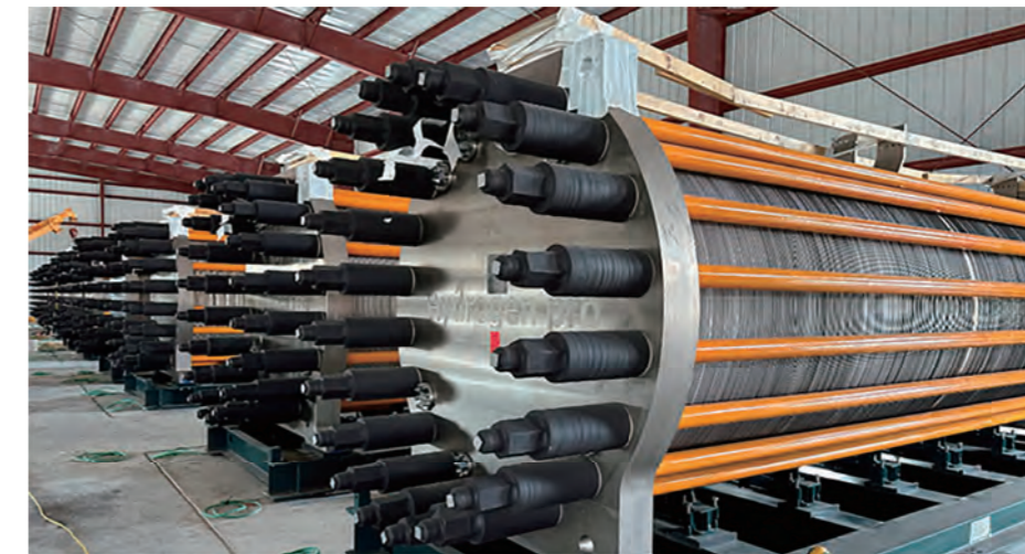
Figure 31 HydrogenPro water electrolysis system
