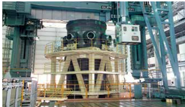
Super Miller - Large-scale, Precision Machine Tool for Reactor Vessel Machining
