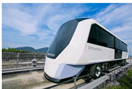
High-speed AGT system achieves a maximum speed of 120 km/h
