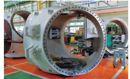
Three blades are attached to this framework.
