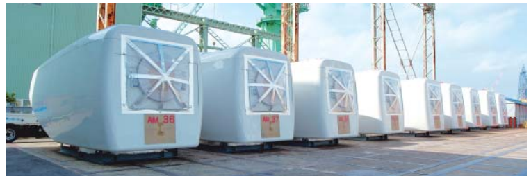
Nacelles, installed atop the turbine tower, contain the generator, rotor, etc.
