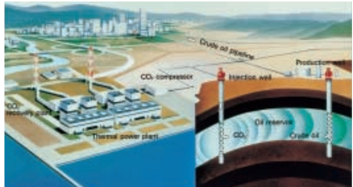
Underground retention system
