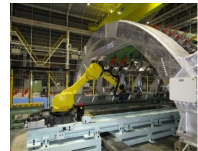
777X automated assembly equipment
