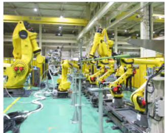
Hiroshima Machinery Works Eba Plant 777X automated assembly line
