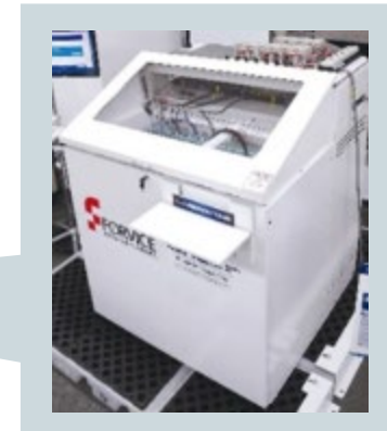
Immersion cooling system
