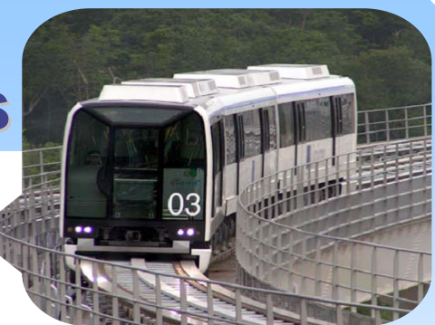
HSST: Electromagnetically Levitated System
