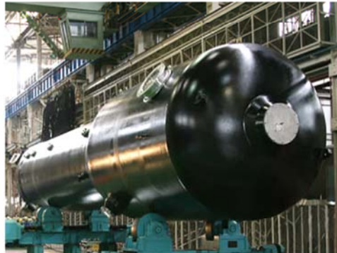
Steam generator replacement
