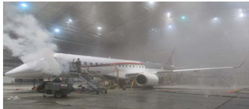
Blowing Snow and Freezing Fog Test (McKinley Laboratory)
