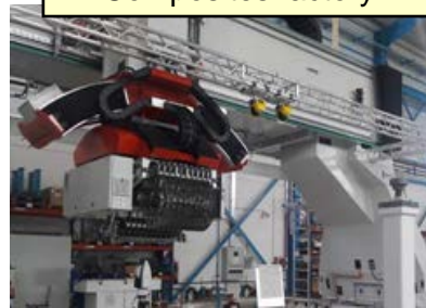
Next Generation Composite Lay up Machine
