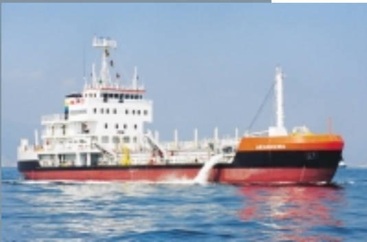
1,000 Trailing Suction Hopper Dredger, H.V. "ARUANGWA"
