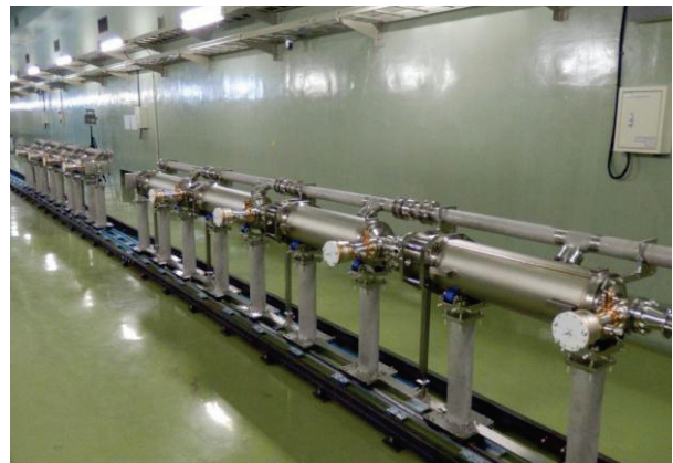
Figure 2: STF cavities with jackets governing high pressure gas safety law in Japan.
