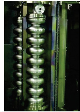
Figure 4: Welding 2 cavities in one batch.
