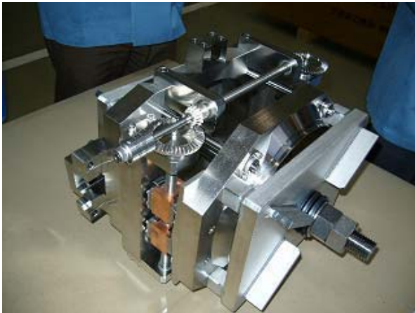
Figure 3: The frequency tuner with test stand.
