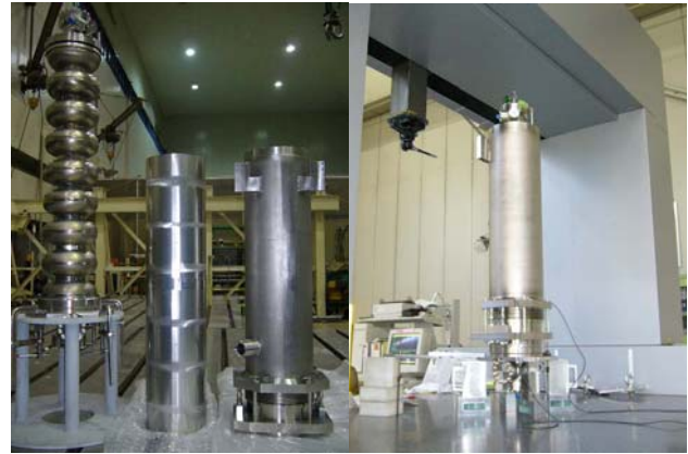
Figure 4: Before and after welding of a helium jacket. A magnetic shield (center left) was placed inside a helium jacket.
