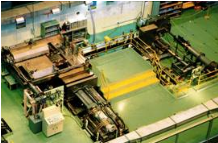
Spend nuclear fuel assembly shearing technologies
