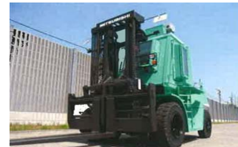
Large, special forklift trucks with shielded cabin
