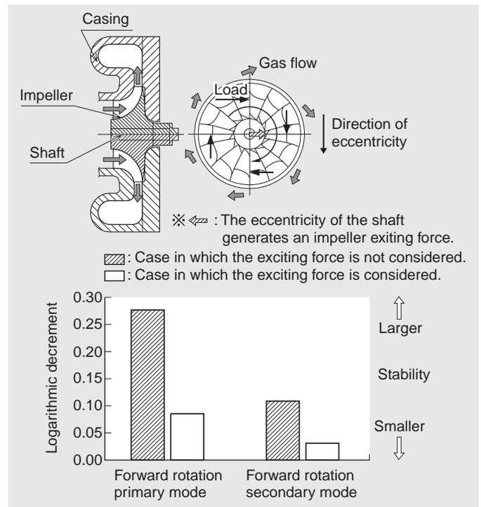
Fig. 3 Comparison of change in shaft system vibration stability depending on existence of impeller exciting force
