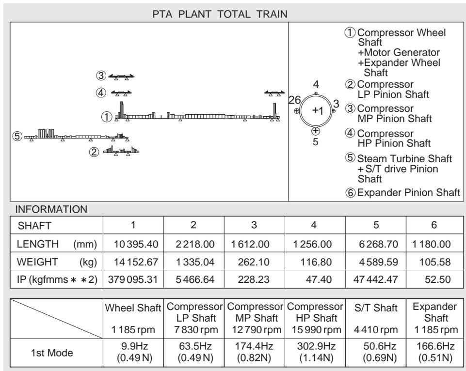
**Fig. 7 Analysis of torsional vibration of compressor train for a PTA plant**
