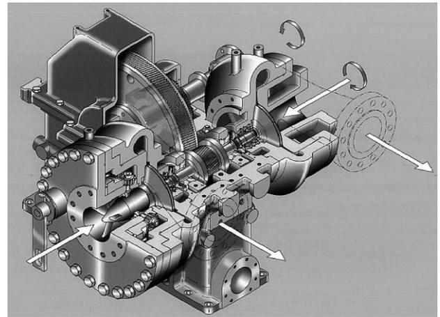
**Fig. 9 Fuel gas geared compressor**
