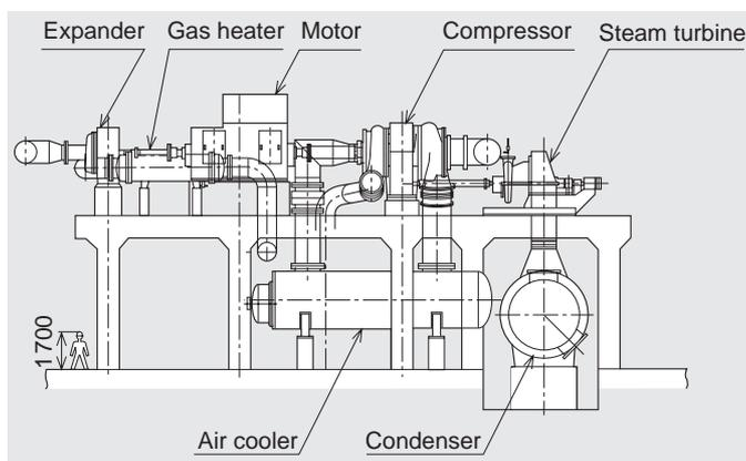
**Fig. 6** Compressor train for a 500 000 tons/year PTA plant
