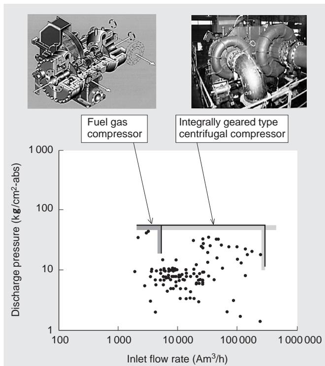
**Fig. 1** Scope of application of geared compressors
