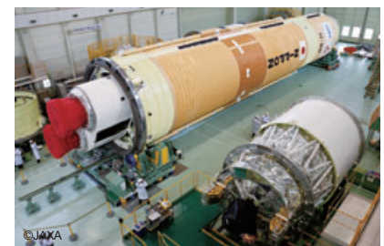
Manufacture of core fuselage for H-IIB Launch Vehicle No. 3
