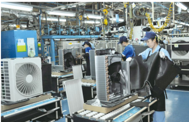
Assembling air-conditioner outdoor units
