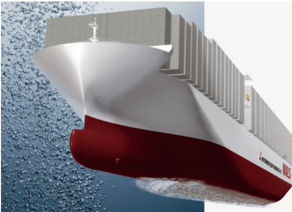
Creating a layer of air between the hull of the ship and the surrounding water reduces frictional drag on the hull.
