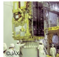
Joining IBUKI and a small sub-satellite with the satellite separation unit
