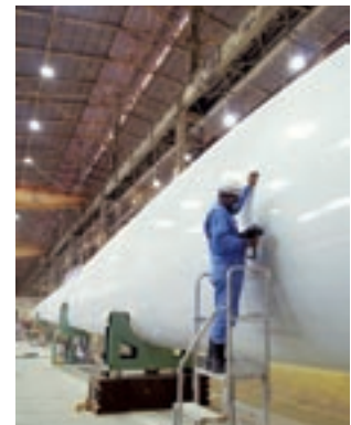
Ultrasonic (nondestructive) blade testing
