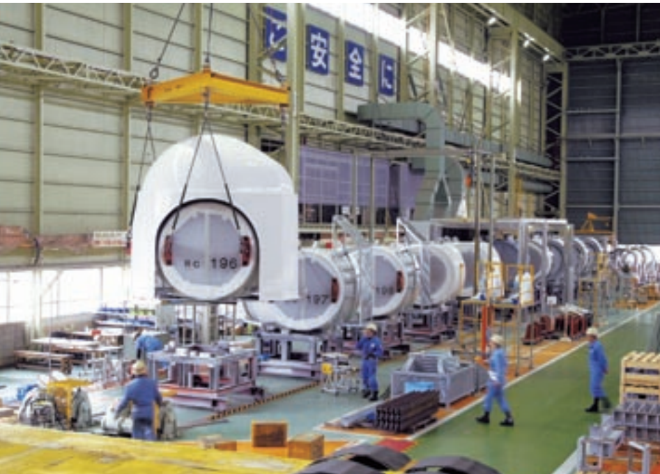
Hub assembly line
