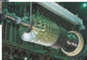
M501G Gas Turbine
