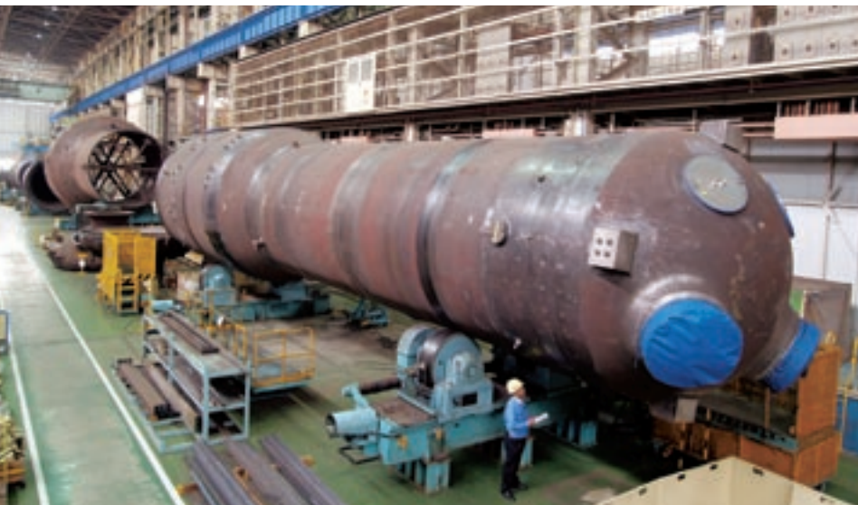
Replacement steam generator under production at the Kobe Shipyard & Machinery Works
