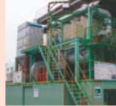
In the carbonization furnace contributing to the improvement of the recycling ratio, No dioxin is generated during the operation of this furnace.
