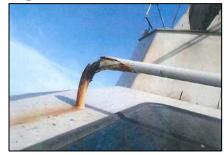
[Progress of corrosion, breakage of wiper]
