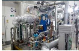
Joint research with the National Institute of Advanced Industrial Science and Technology achieved stable combustion with 100% hydrogen
