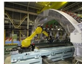
777X automated assembly equipment
