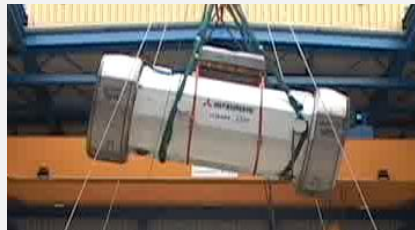
Cask (drop test of real equipment)
