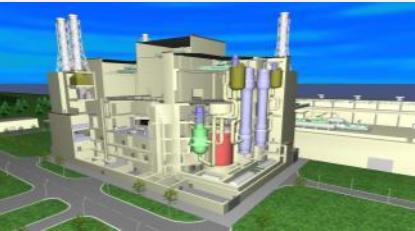
Commercial reactor (practical application of FBR)
