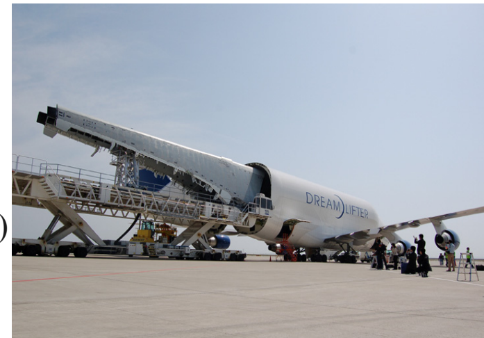
The wing loaded into Boeing Dreamlifter at Central Japan International Airport for air transportation
