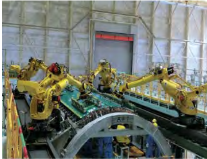
Automated 777X assembly line
