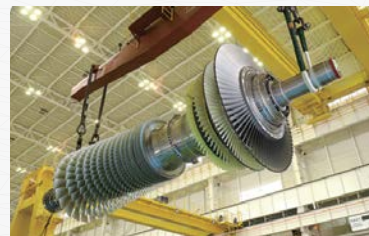
A "J-Series" gas turbine achieved the world's highest turbine inlet temperature, 1,600°C, during verification testing. (2011)
