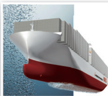
▲ Mitsubishi Air Lubrication System (MALS)
