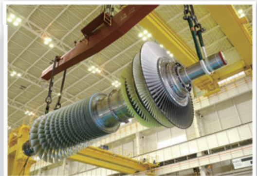
▲ M501J gas turbine
